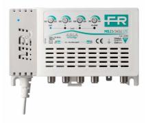
**3 input (FM+III+DAB, UHF) multiband TV indoor amplifier** with 32dB gain and output level up to **120dBµV in UHF band**, separate amplification, independent level adjustment (20dB) for each input and low noise figure. **Built-in 694MHz 5G and 4G LTE filter.**
